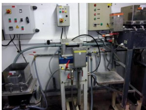
\*Note: the 10/100 mm slotted plate retains the possible remaining unwanted materials not previously removed indicating a possible insufficient quality of the pulp suspension. It is used as a monitoring device to evaluate the removal efficiency of previous screening steps.
