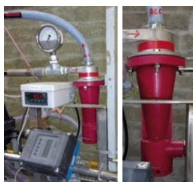
The cleaning step is carried out under industrial conditions with limited rejects flow rate to minimise fibre losses. Indeed, heavyweight cleaners can be very effective but with a limited selectivity: rejects are composed with the unwanted materials but also with some cellulosic fibres.
